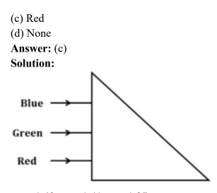
$\mu_B = 1.49, \mu_G = 1.41, \mu_R = 1.27$ Incident angle = i, Critical angle =  $i_c$  $i > i_c$  (Total internal reflection will take place)
